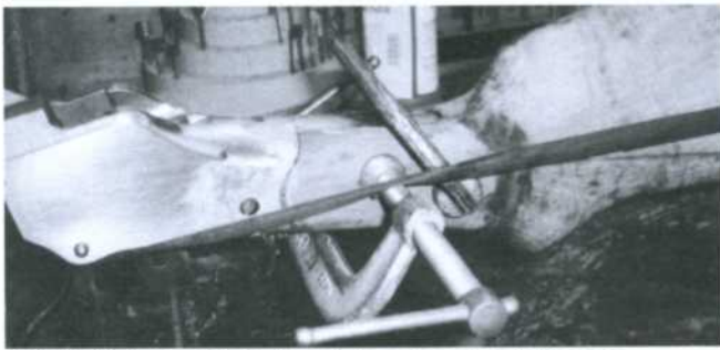
High Wall stock with the break Acraglased and clamped.
