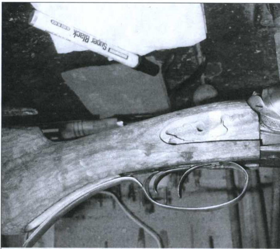
Above: The trigger guard loop has been opened up allowing full movement of the rear trigger.
